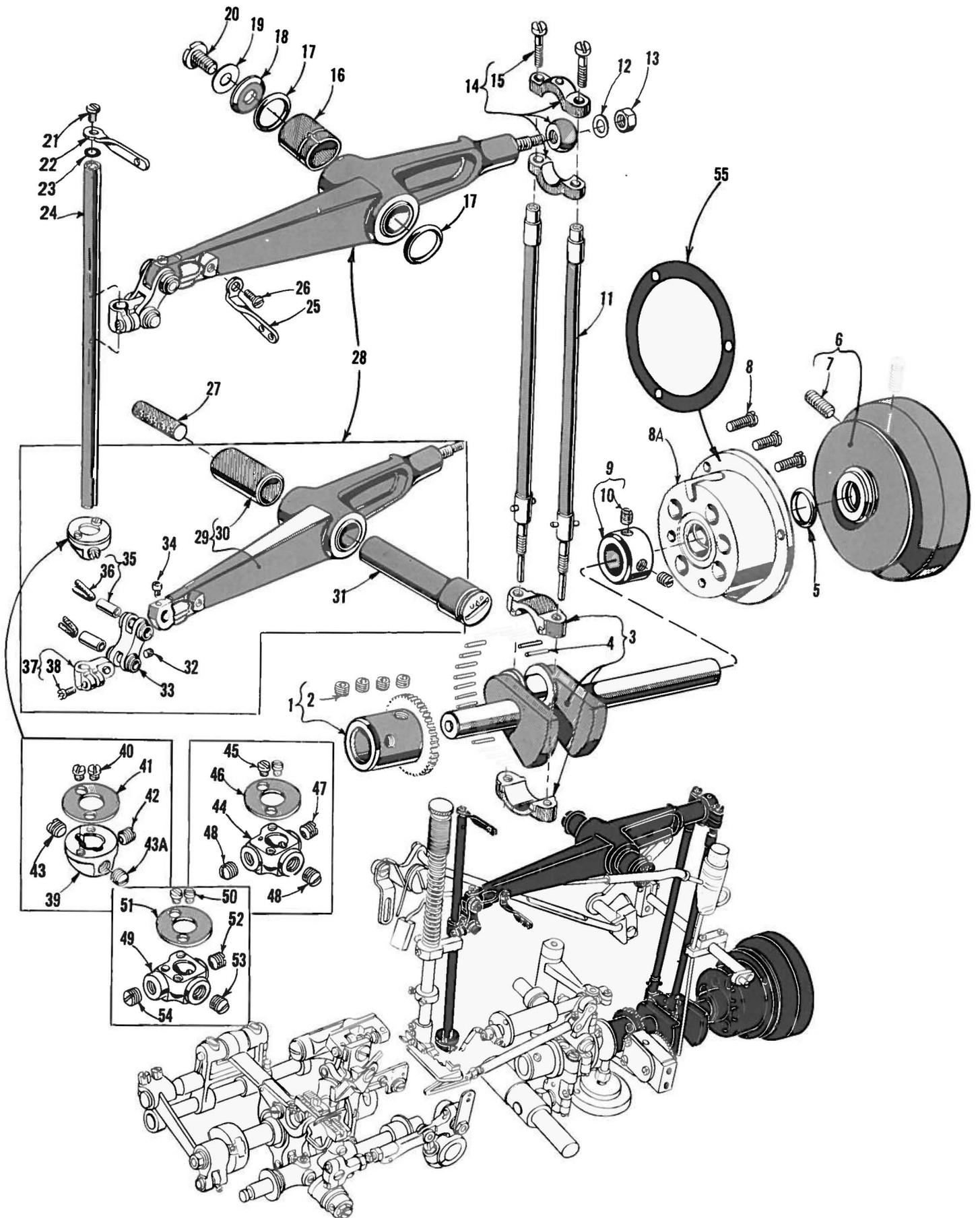
CRANKSHAFT, NEEDLE LEVER, NEEDLE BAR AND NEEDLE HEADS
