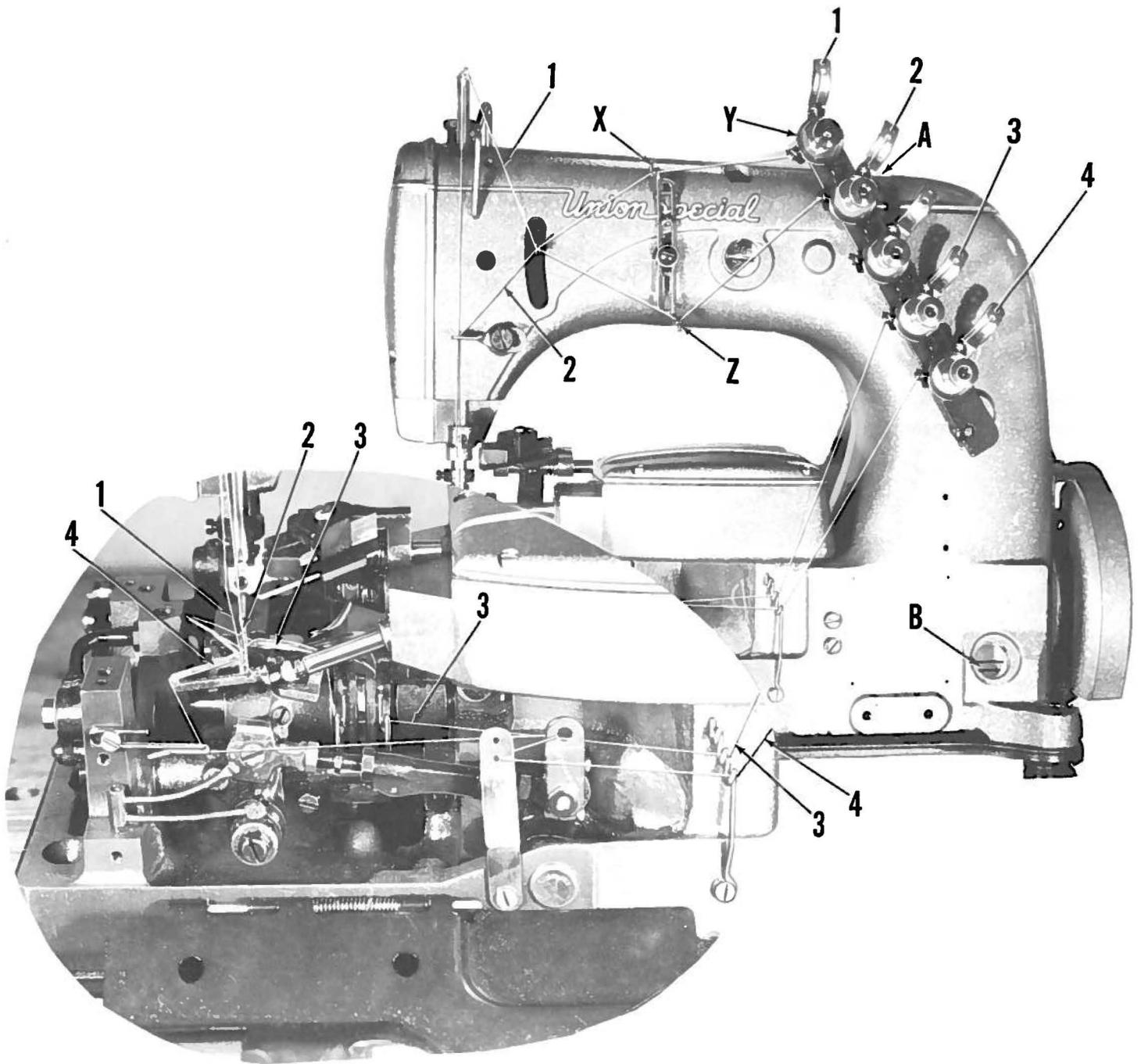
OILING AND THREADING DIAGRAM FOR CLASS 52300 MACHINES
