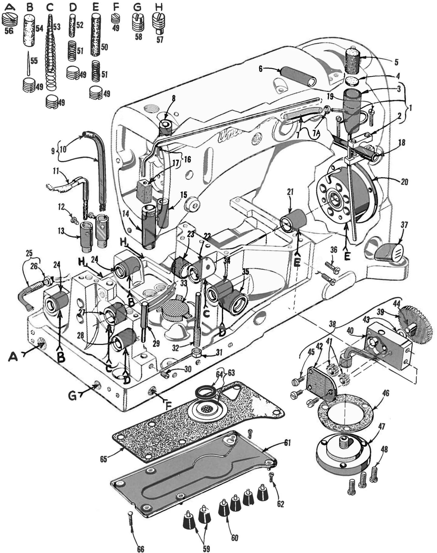
MAIN FRAME, BUSHINGS AND MISCELLANEOUS OILING PARTS
