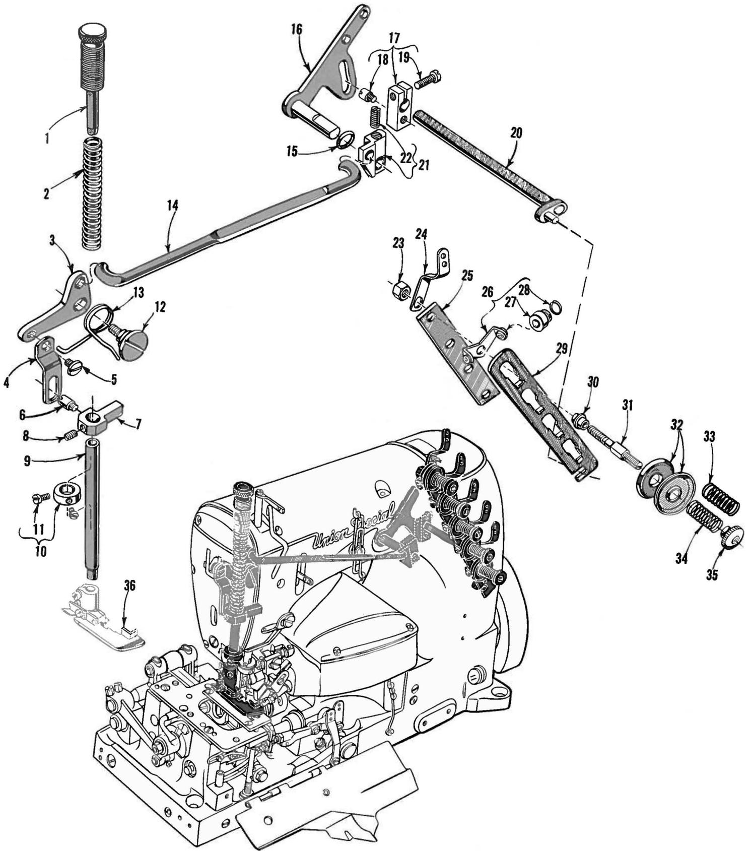
THREAD TENSION AND LIFTER LEVER PARTS
